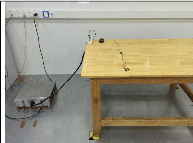
Conducted Emissions Test Setup Front View
