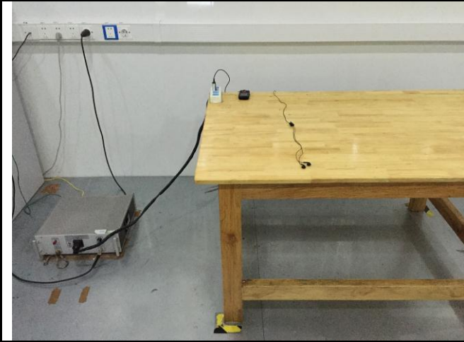
Conducted Emissions Test Setup Front View
