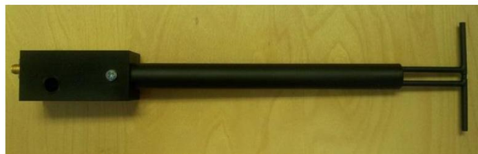
Figure 1 – MVG COMOSAR Validation Dipole
