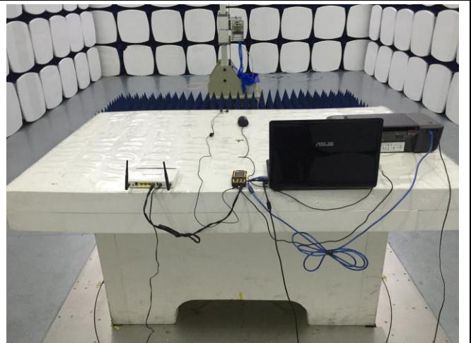
Radiated Emissions Test Setup Above 1GHz
