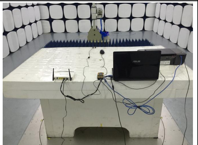
Radiated Emissions Test Setup Above 1GHz
