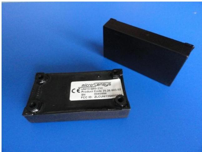
The RFID read/write module UNI13-Q60 is part of the inductive read/write- identification system iID®3000 and serves for the reading and writing of 13.56MHz RFID transponders. It supports RFID transponder systems like iID®, TELID®, ISO15693, I-CODE™, tag-it™, my-D™, LEGIC® and further. The UNI16-Q60 is available in two types, with a serial interface and with a USB interface to the host computer.
