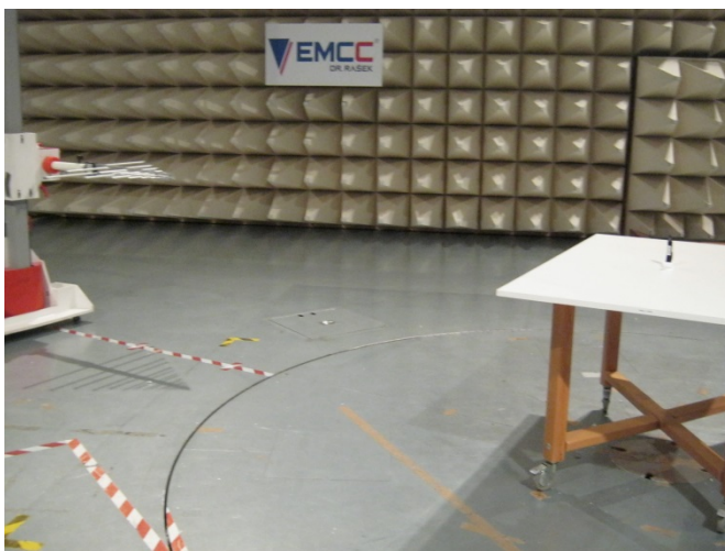
Radiated emissions measurement at 3 m distance 300 MHz – 1000 MHz
