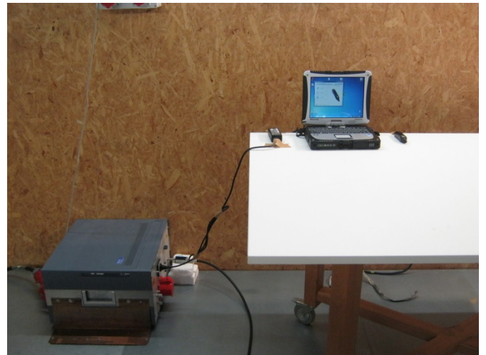
Conducted emissions measurement 150 kHz – 30 MHz
