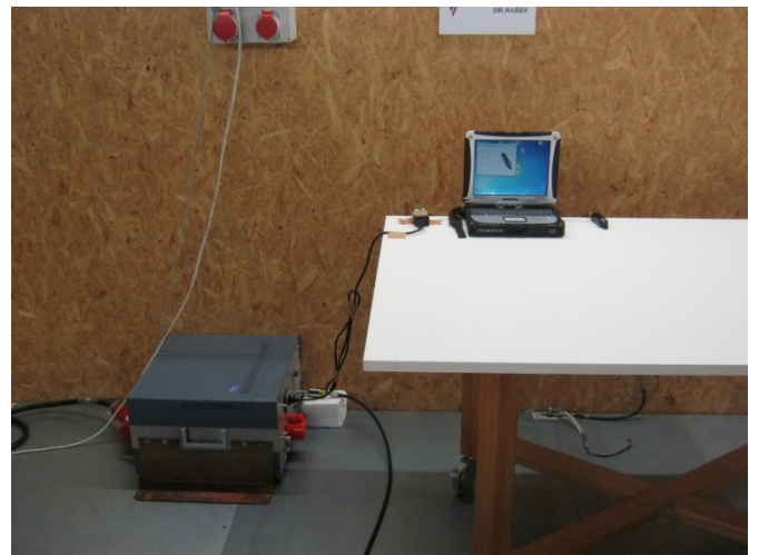
Conducted emissions measurement 150 kHz – 30 MHz
