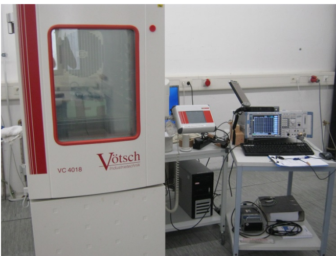
Test setup frequency stability over temperature
