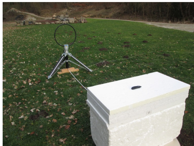
Radiated emissions measurement at 3 m distance at open field site; 9 kHz – 30 MHz
