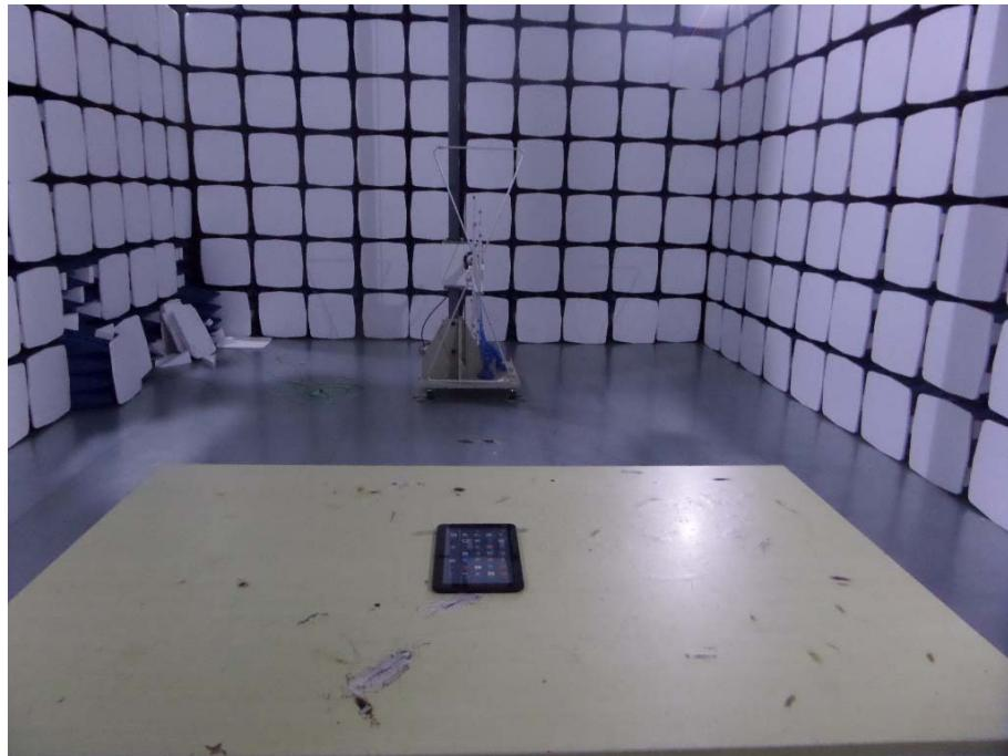
**Radiation Emission Test Setup (Above 1GHz)**
