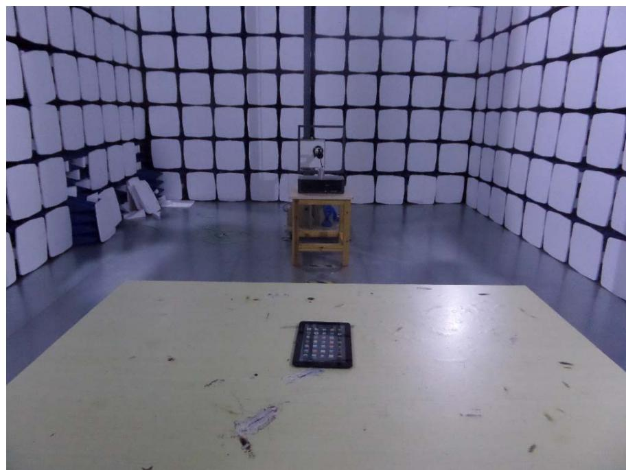
**Radiation Emission Test Setup (30MHz to 1GHz)**
