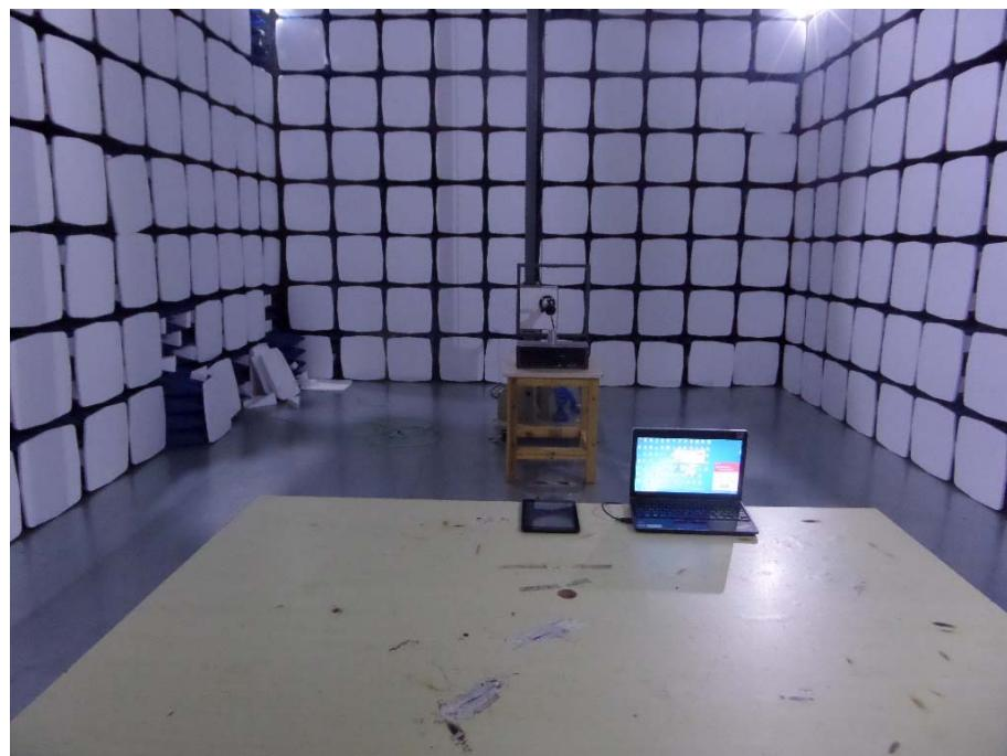
**Radiation Emission Test Setup (Below 30MHz to 1GHz)***Charging & Playing Mode*
