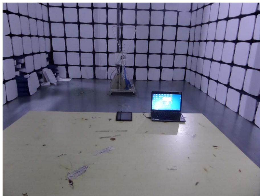
**Radiation Emission Test Setup (Above 1GHz)***Charging & Playing Mode*
