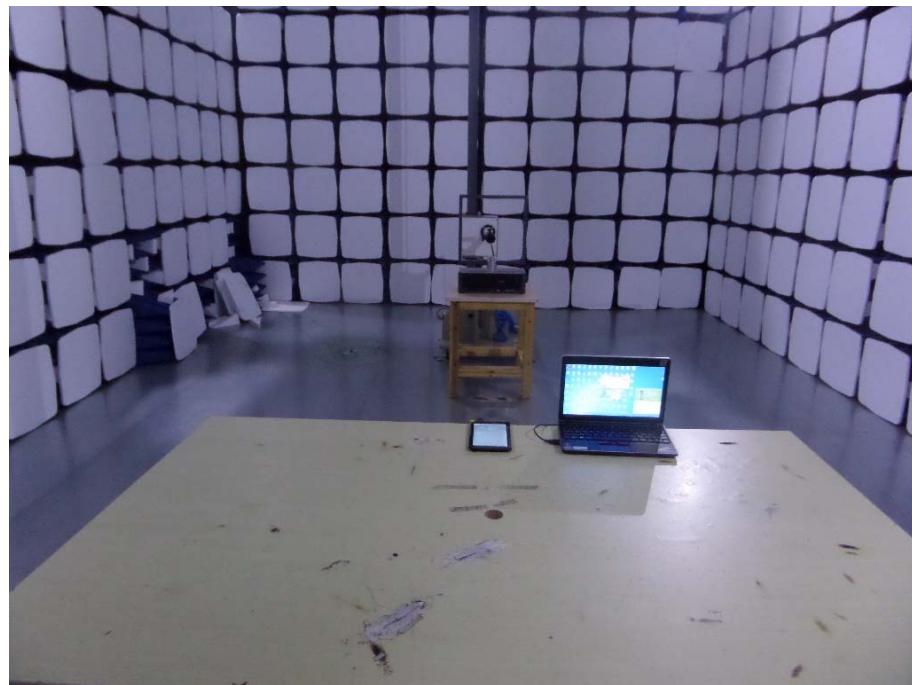
**Radiation Emission Test Setup (Below 30MHz to 1GHz)***Charging & Playing Mode*
