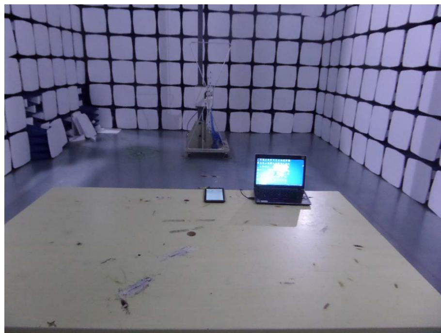
**Radiation Emission Test Setup (Above 1GHz)***Charging & Playing Mode*
