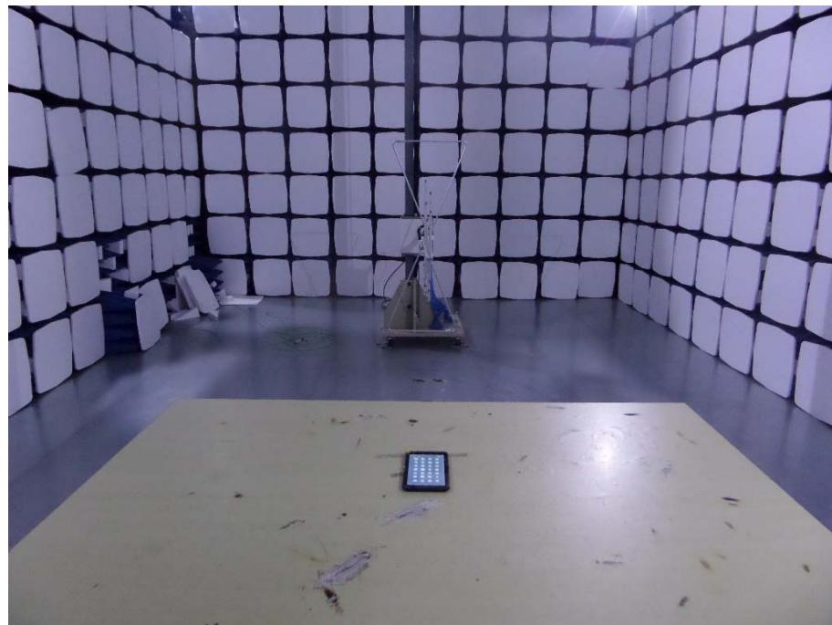
**Radiation Emission Test Setup (Above 1GHz)**
