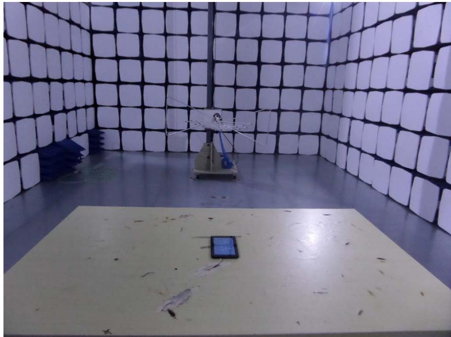
**Radiation Emission Test Setup (Above 1GHz)**
