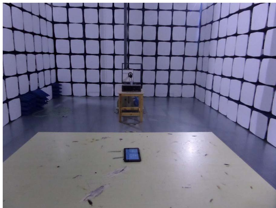
**Radiation Emission Test Setup (30MHz to 1GHz)**
