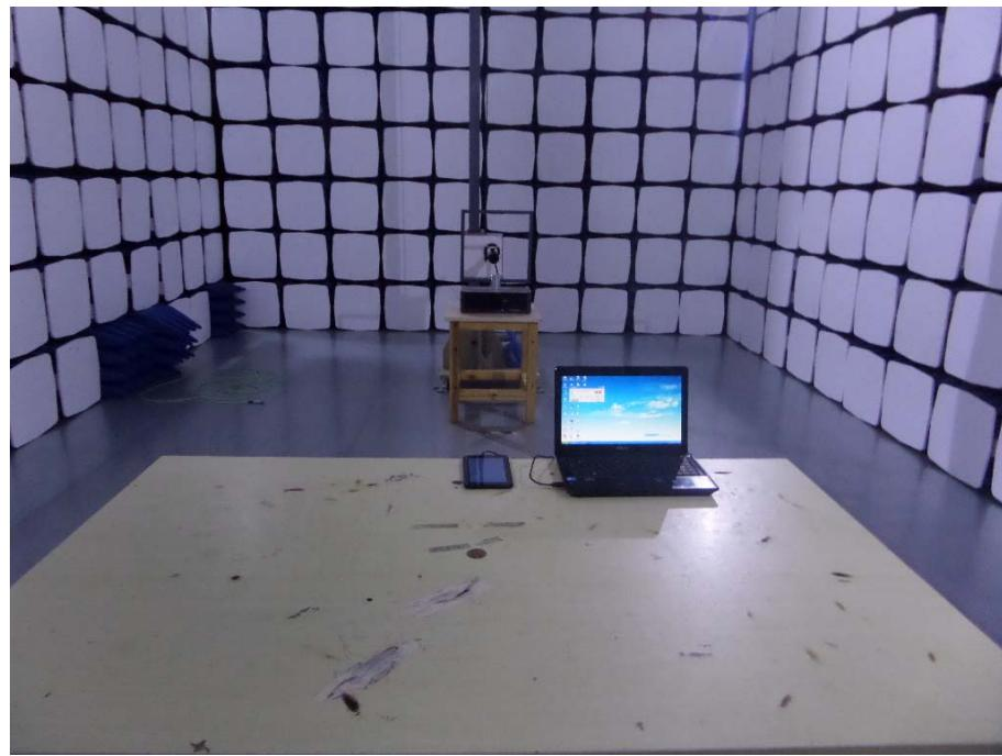
**Radiation Emission Test Setup (Below 30MHz to 1GHz)***Charging & Playing Mode*
