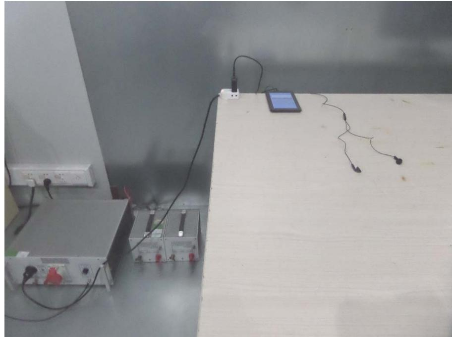
**Radiation Emission Test Setup (Below 30MHz)***Charging & playing mode*
