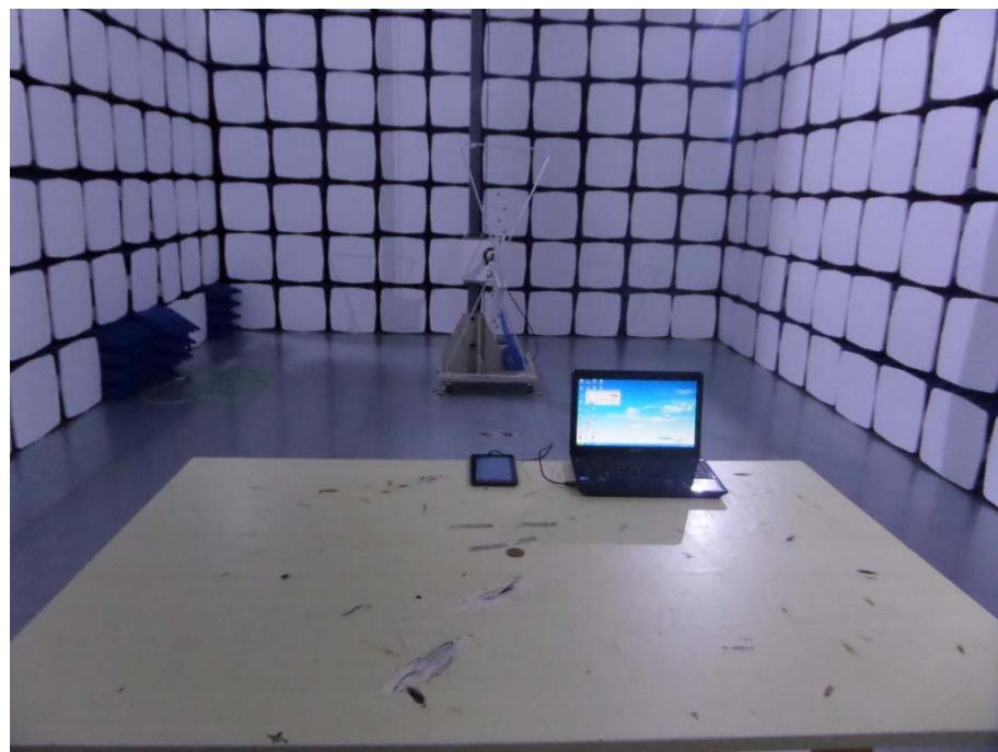
**Radiation Emission Test Setup (Above 1GHz)***Charging & Playing Mode*
