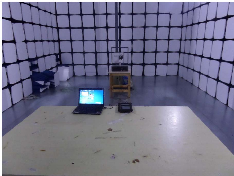
**Radiation Emission Test Setup (Below 30MHz to 1GHz)**
