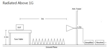
Radiated emission tests were performed in the 3 meters chamber test site, using the setup accordance with the ANSI C63.10-2013. The specification used was the FCC Part 15.209 and FCC 15.247 Limits.
