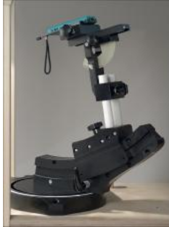
Fig. 15-4 Device Holder for Transmitters
