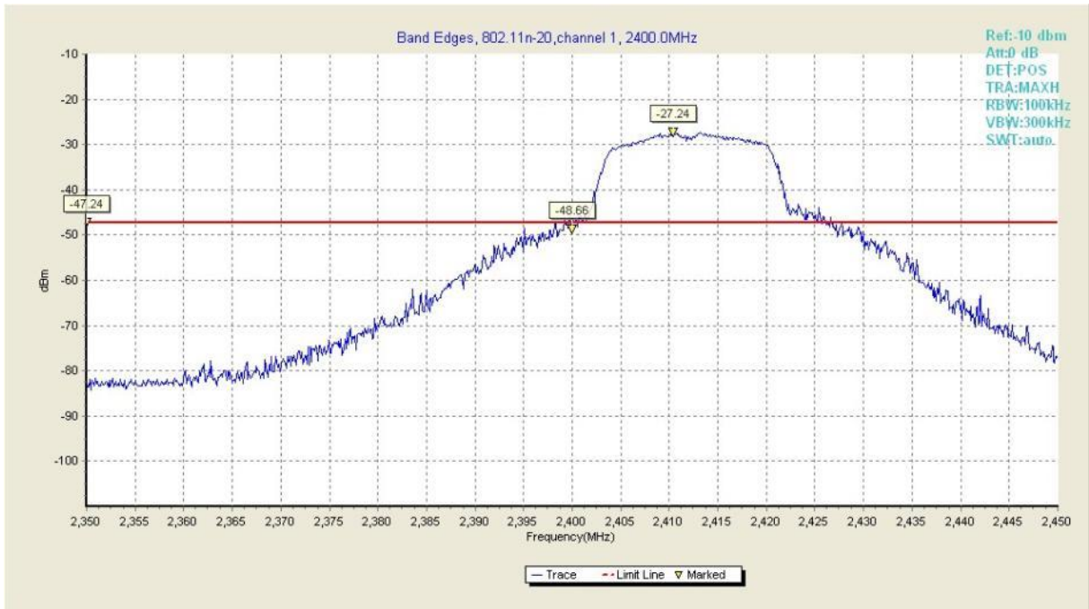
Fig29. Frequency Band Edges of 802.11n-20 in channel 1,2400MHz
