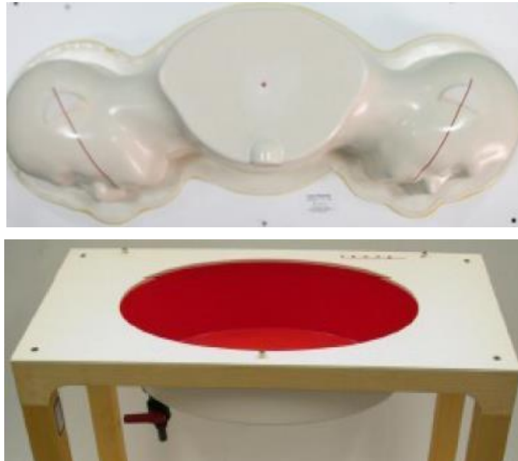
Figure 6 SAM Twin Phantom and ELI Phantom
