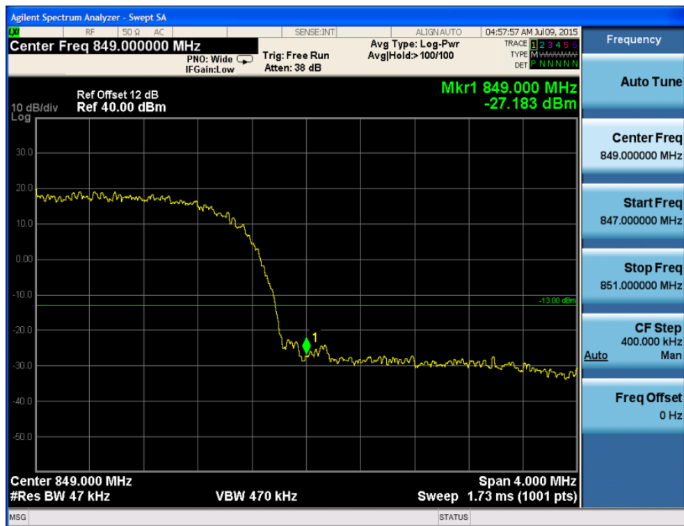
Fig.40 WCDMA Band V-CH4232 Band Edge Compliance HSDPA Subtest 1
