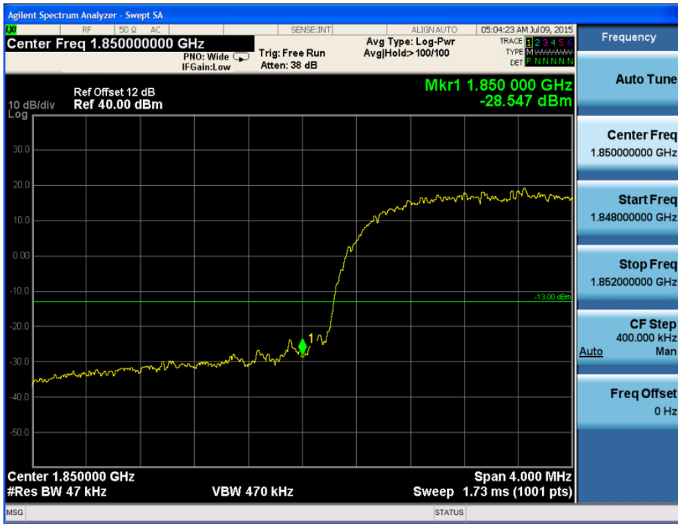
Fig.47 WCDMA Band II-CH9263Band Edge Compliance HSUPA Subtest 5
