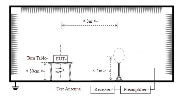
2) For radiated emissions from 30MHz to1GHz
