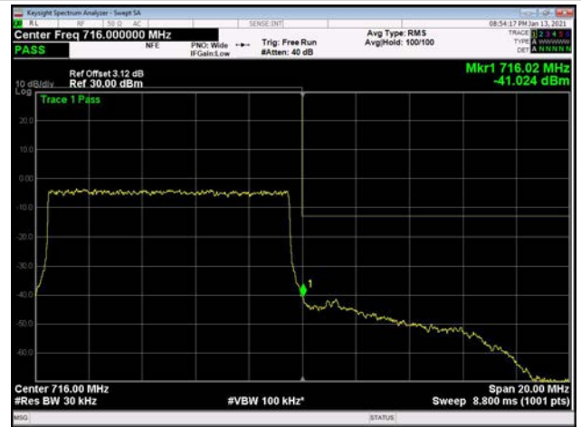
10MHz / 64QAM / High Channel / 1 RB
