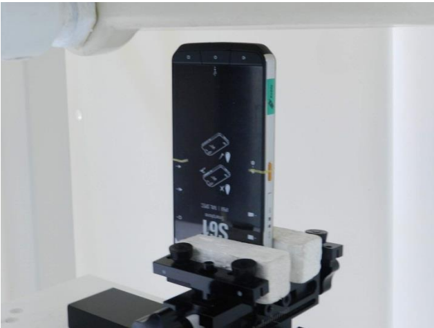
Bottom Side, Test Separation 10 mm
