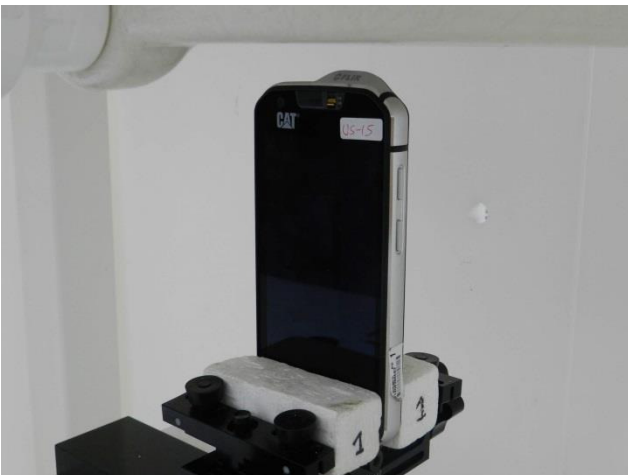
Top Side, Test Separation 10 mm
