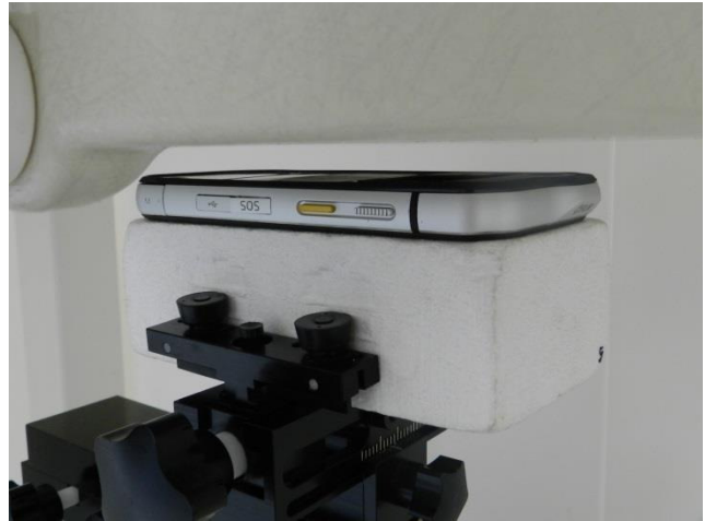
Back, Test Separation 10 mm
