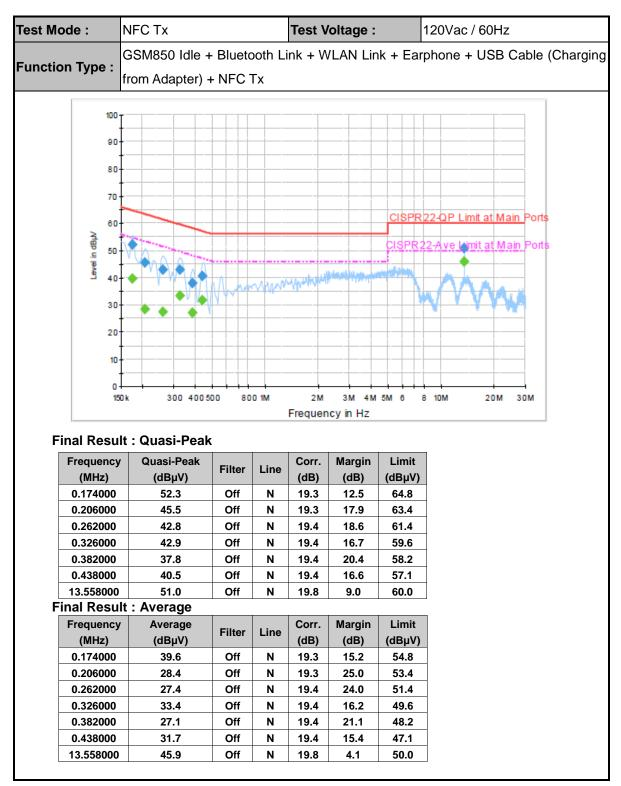
Remark: 13.558MHz is the NFC RF fundamental signal.
