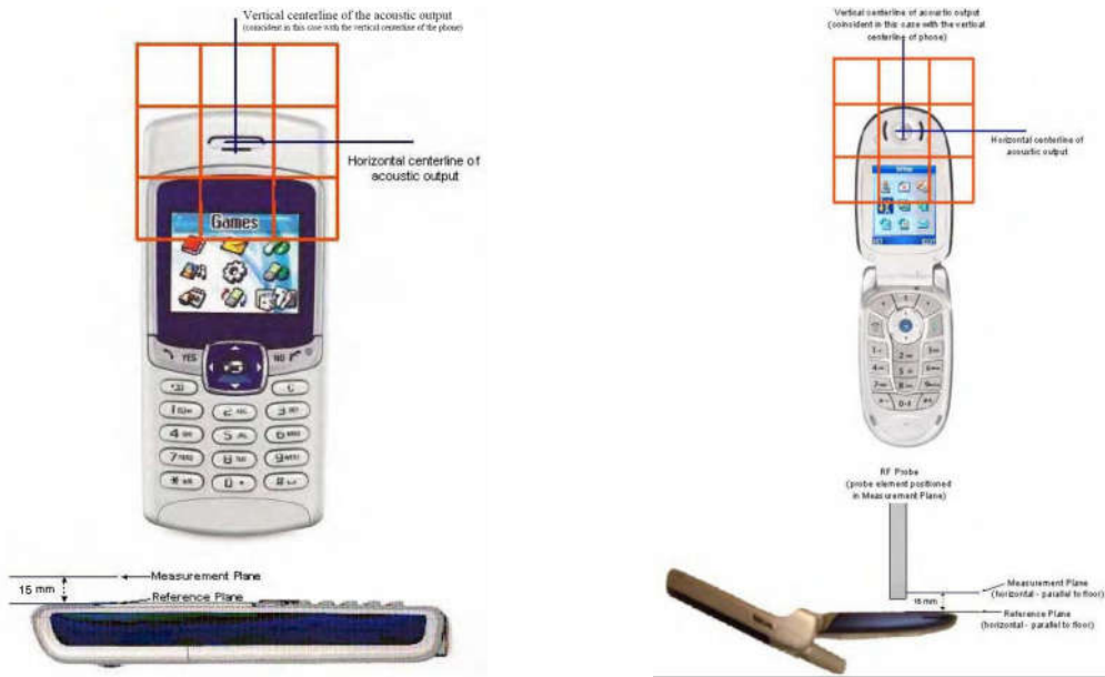
Fig 8.2 EUT reference and plane for HAC RF emission measurements
