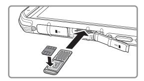
4. Insert the SIM tray into the SIM card slot and close the SIM door.
