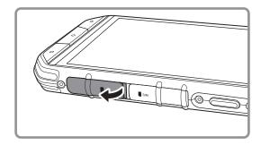
2. Insert a microSD card into the memory card slot with gold contacts facing up.
