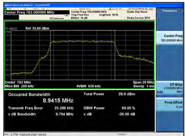
Band13 / 10MHz / High CH / 16QAM
