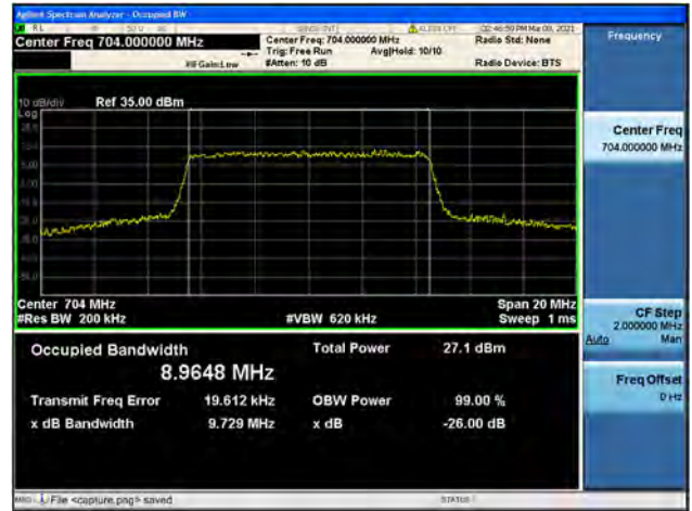
Band12 / 10MHz / Mid CH / 16QAM
