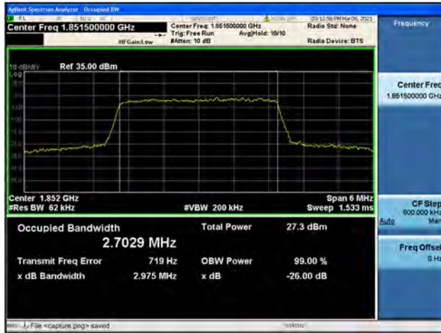
Band25 / 3MHz / Mid CH / QPSK
