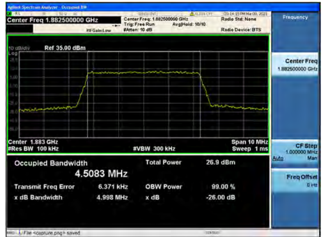
Band25 / 5MHz / High CH / 16QAM
