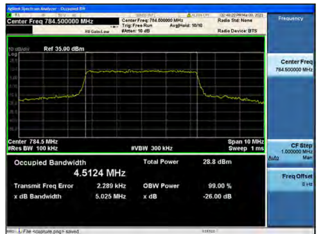
Band13 / 5MHz / High CH / 16QAM
