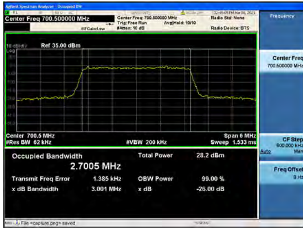
Band12 / 3MHz / Mid CH / QPSK
