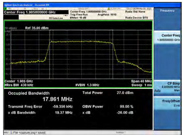
Band25 / 20MHz / High CH / 16QAM
