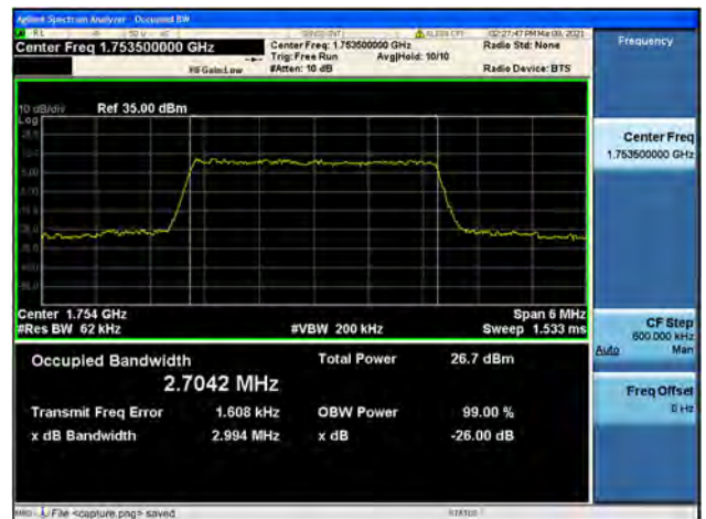
Band4 / 3MHz / High CH / 16QAM
