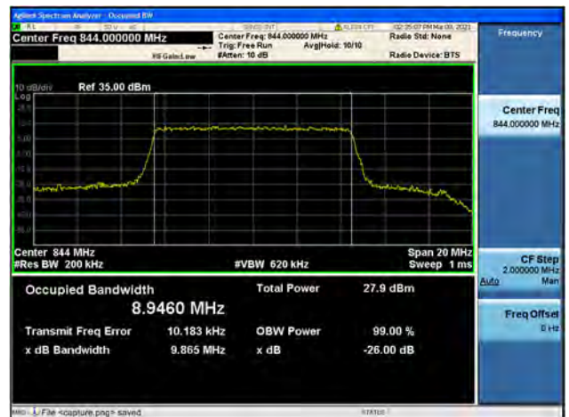
Band5 / 10MHz / High CH / 16QAM
