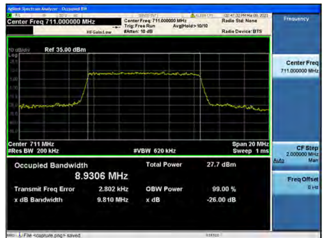
Band12 / 10MHz / High CH / 16QAM
