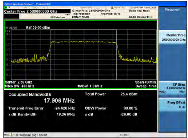
Band38 / 20MHz / Mid CH / 16QAM
