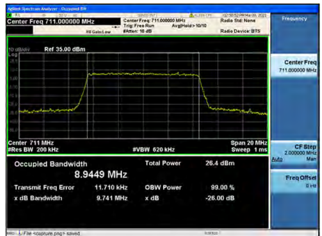
Band17 / 10MHz / High CH / 16QAM
