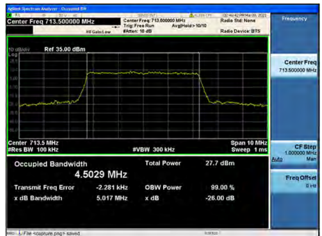
Band12 / 5MHz / High CH / 16QAM
