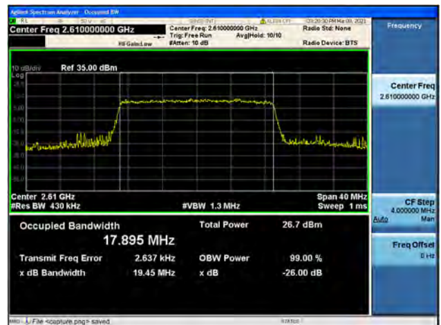
Band38 / 20MHz / High CH / 16QAM
