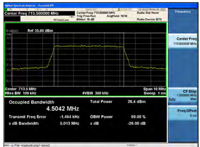
Band17 / 5MHz / High CH / 16QAM
