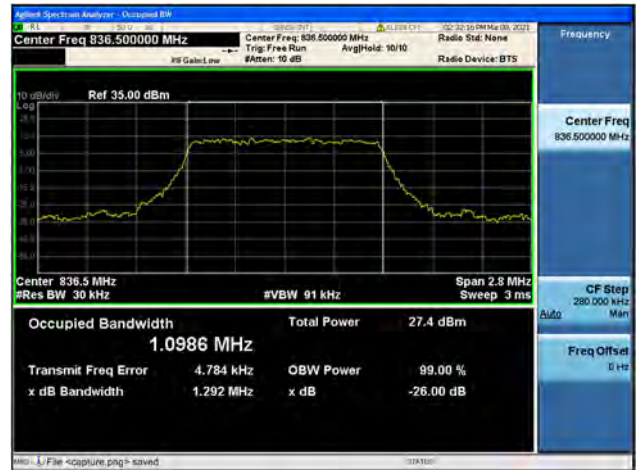
Band5 / 1.4MHz / High CH / 16QAM
