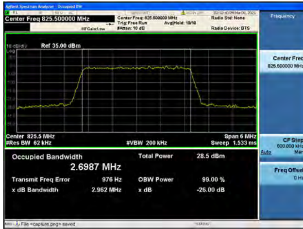
Band5 / 3MHz / Mid CH / QPSK
