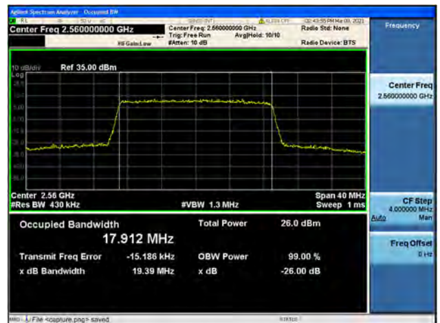
Band7 / 20MHz / High CH / 16QAM
