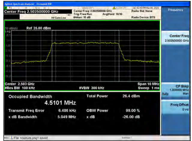
Band7 / 5MHz / Mid CH / 16QAM
