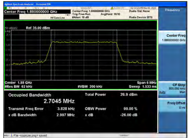
Band2 / 3MHz / High CH / 16QAM
