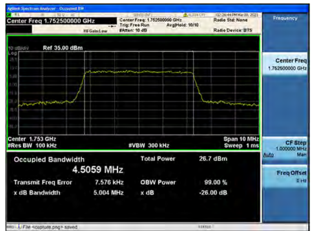
Band4 / 5MHz / High CH / 16QAM
