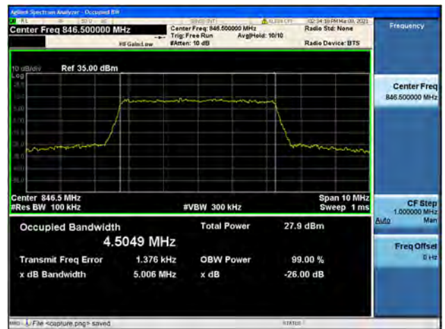
Band5 / 5MHz / High CH / 16QAM
