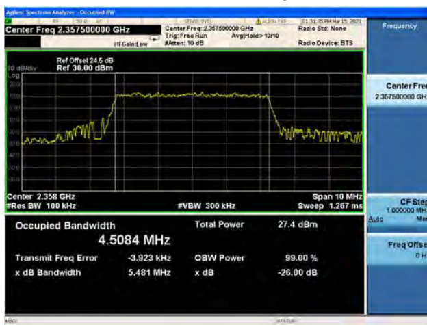
Band40/ Block B / 5MHz / High CH / QPSK
