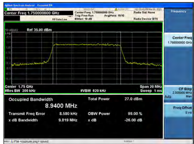
Band4 / 10MHz / High CH / 16QAM
