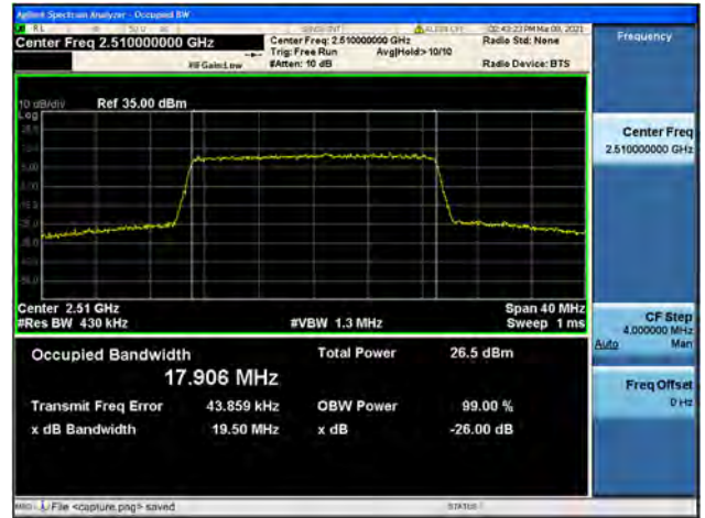
Band7 / 20MHz / Mid CH / 16QAM
