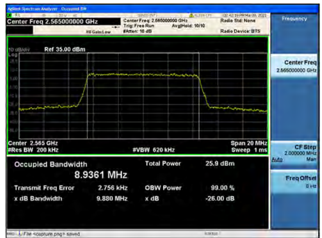
Band7 / 10MHz / High CH / 16QAM
