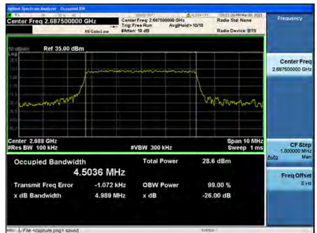
Band41 / 5MHz / High CH / 16QAM
