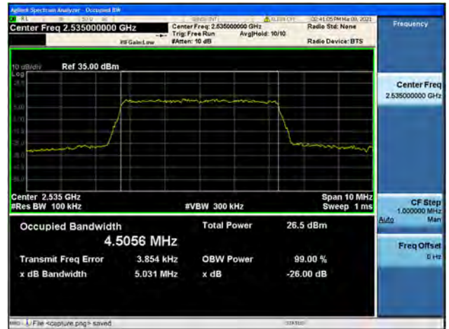
Band7 / 5MHz / High CH / 16QAM
