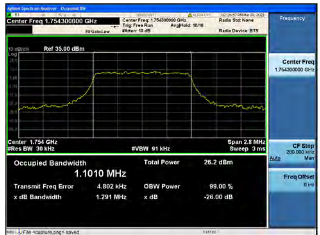
Band4 / 1.4MHz / High CH / 16QAM
