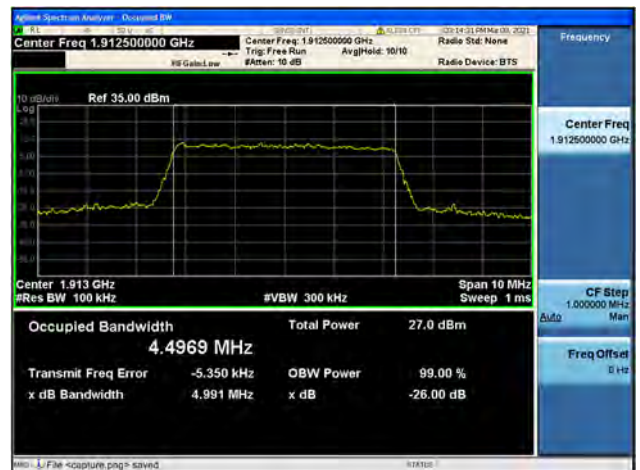
Band25 / 5MHz / High CH / 16QAM
