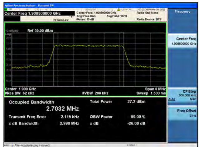
Band2 / 3MHz / High CH / 16QAM
