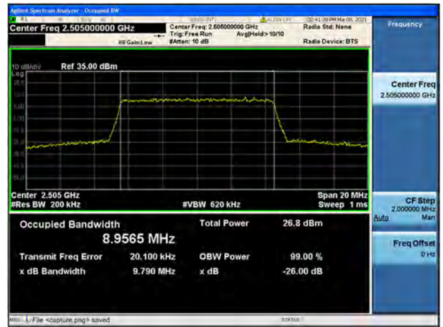
Band7 / 10MHz / Mid CH / 16QAM
