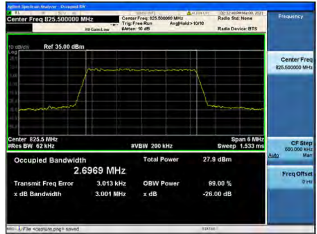
Band5 / 3MHz / Mid CH / 16QAM
