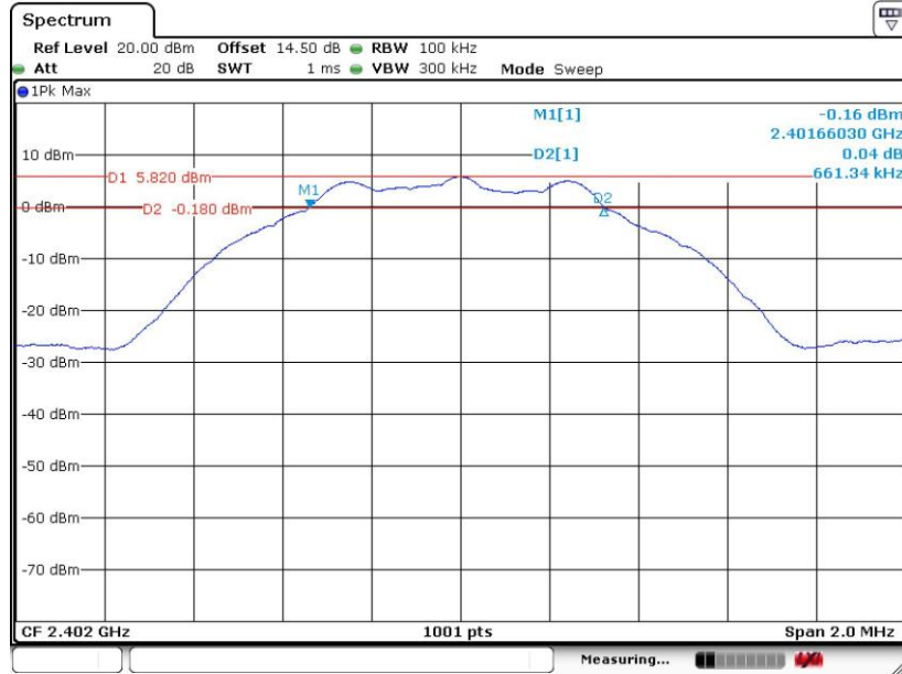
6 dB Bandwidth Plot on Channel 00
