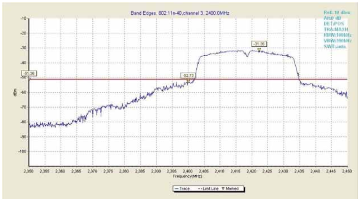
Fig31. Frequency Band Edges of 802.11n-40 in channel 1,2422MHz
