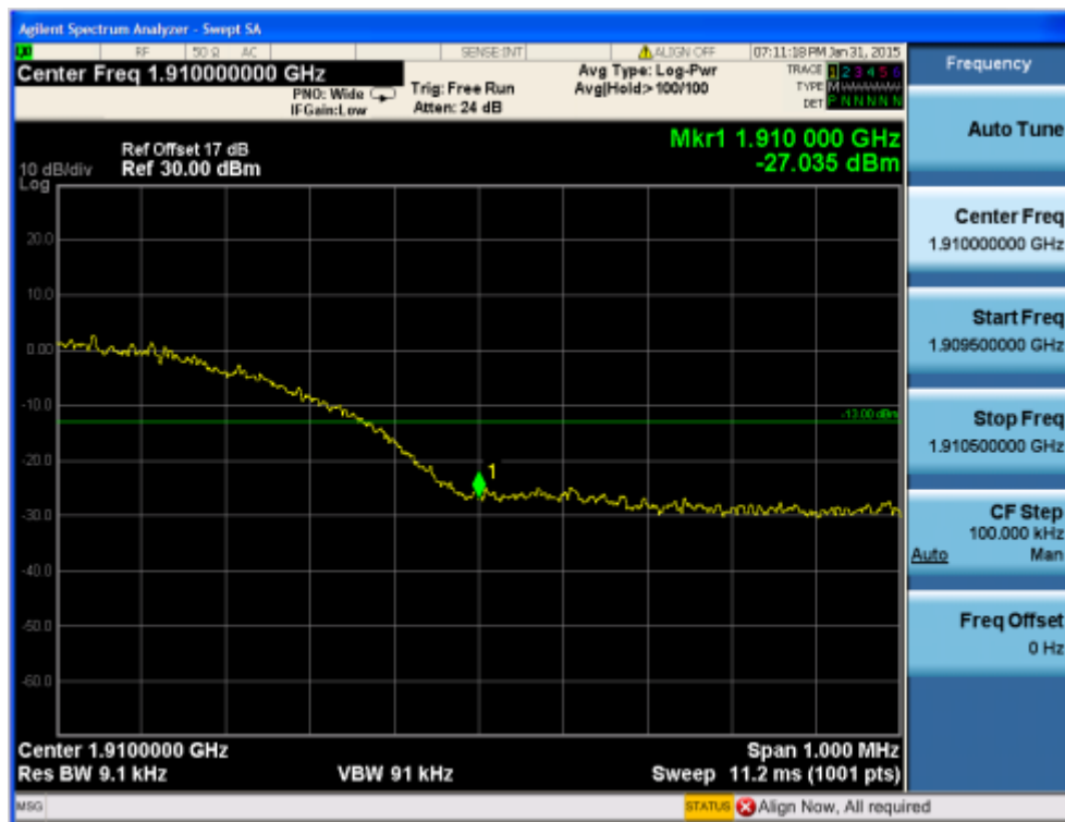
Fig.44 WCDMA Band II-CH9538 Band Edge Compliance
