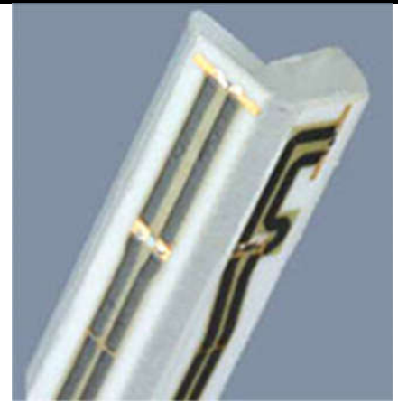
Fig 5.2 Photo of E-field Probe
