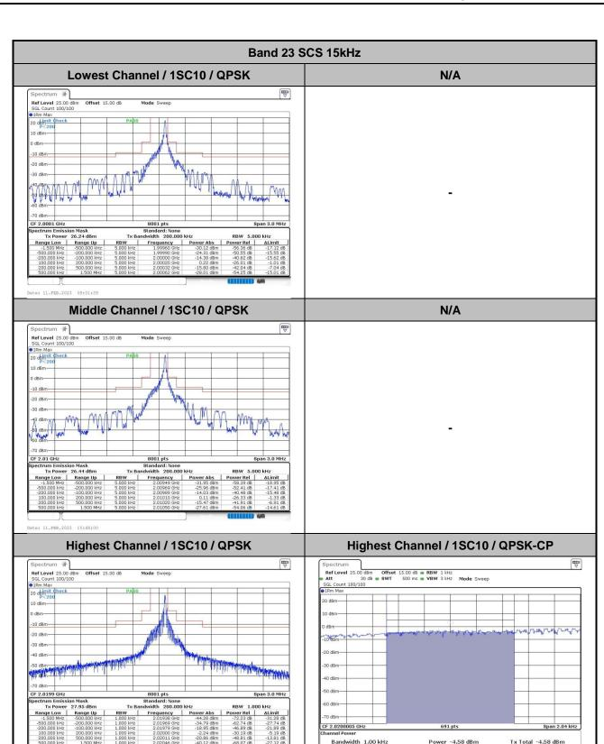
Remark: The above results of RBW 1kHz corrected by 10log(4kHz/1kHz) is passed.
