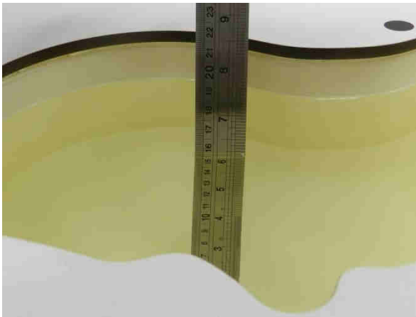
Fig 11.1 Photo of Liquid Height for Head SAR
