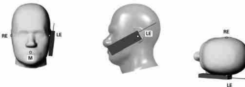
Fig 9.2.3 cheek or touch position. The reference points for the right ear (RE), left ear (LE), and mouth (M), which establish the Reference Plane for handset positioning, are indicated.
