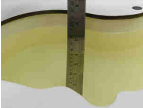
Fig 10.1 Photo of Liquid Height for Head SAR
