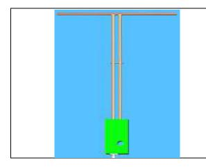
The dipoles used are based on the IEEE-1528 standard, and is complied with mechanical and electrical specifications in line with the requirements of IEEE. the table below provides details for the mechanical and electrical Specifications for the dipoles.
