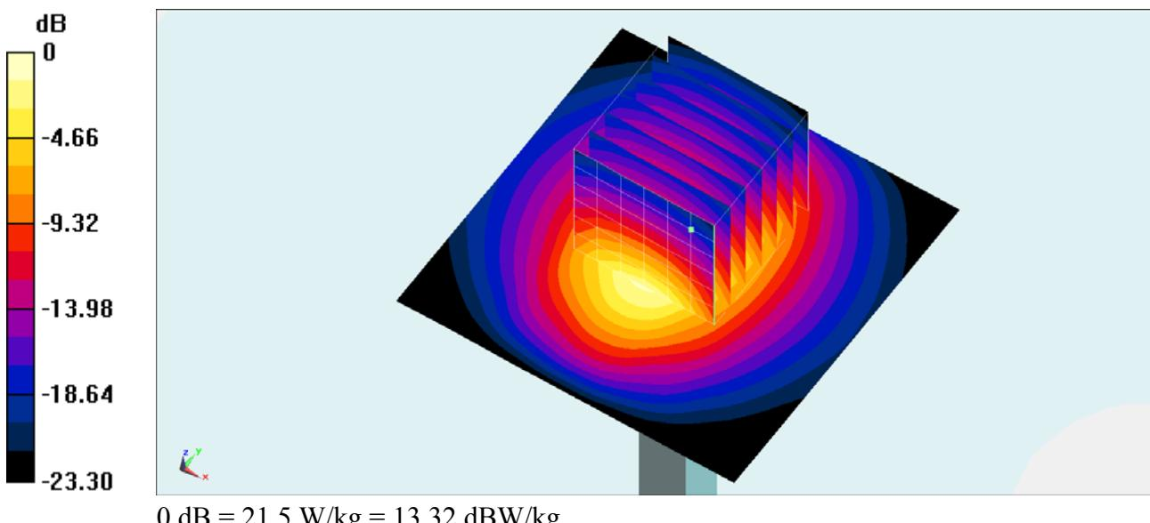
**System Check\_Body\_2450MHz\_130119****DUT: D2450V2-SN:736**
