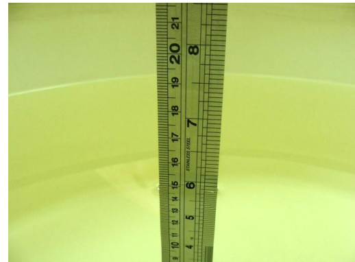
Fig 6.2 Photo of Liquid Height for Body SAR
