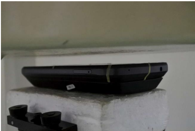
Front With Battery Pack, Test Separation 10 mm
