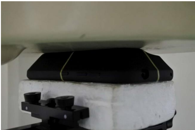
Back With Battery Pack + Holster Test Separation 0 mm
