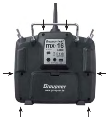
Arrangement of the case back screws
