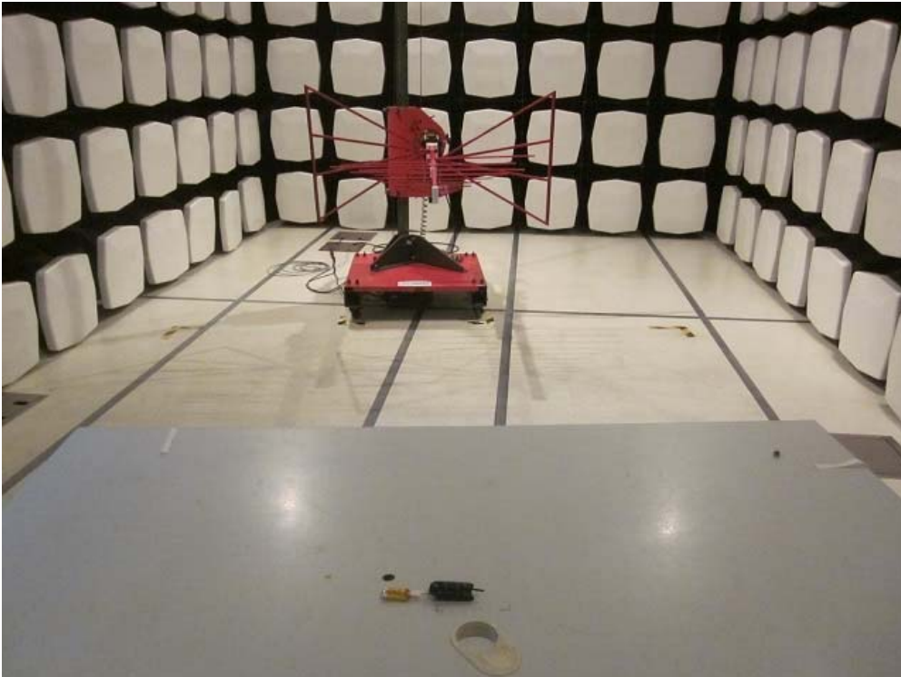
Measurement of Radiated Emission Test Set Up
