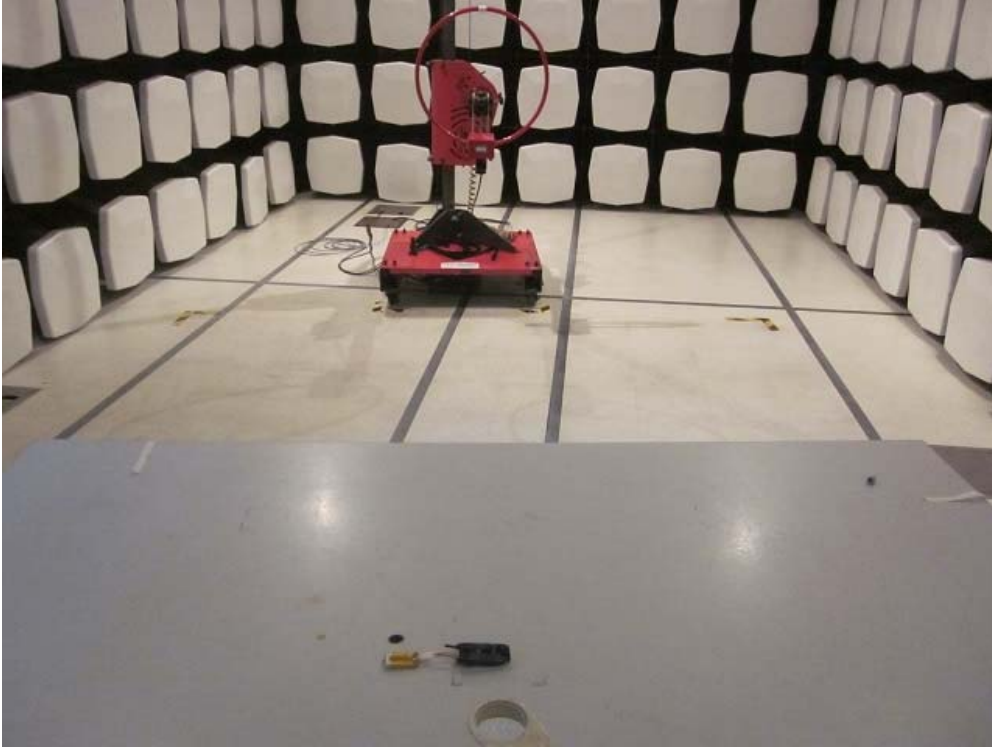
Measurement of Radiated Emission Test Set Up
