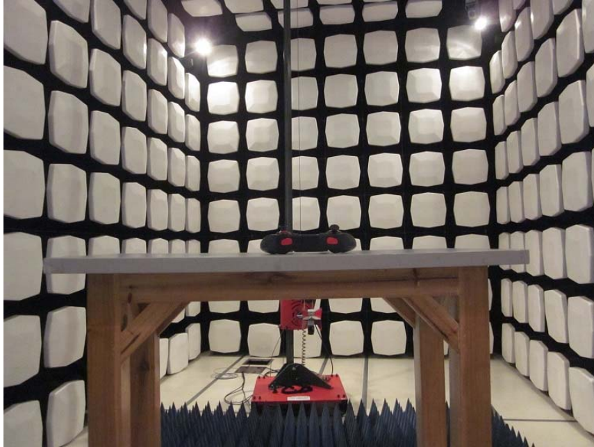
Measurement of Radiated Emission Test Set Up
