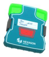
HxGN Mine Personal Alert is the first accident-avoidance device worn by field personnel that ensures visibility around heavy equipment. Using the reliability and precision of Time of Flight technology in the Ultra-Wide Band frequency, Personal Alert is integrated with Hexagon Mining's Collision Avoidance System (CAS) for a comprehensive warning solution.
