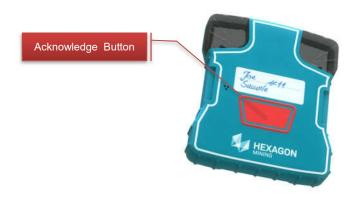
Personnel wearing Pedestrian Tags can silence the Pedestrian tag from threats alerting, this does not acknowledge all other vehicle alarms, but only the sound and vibratory alarms from the current situation once the button is pressed. The personnel will get another alarm if a second vehicle approaches, even if alerts with the first vehicle have already been silenced.
