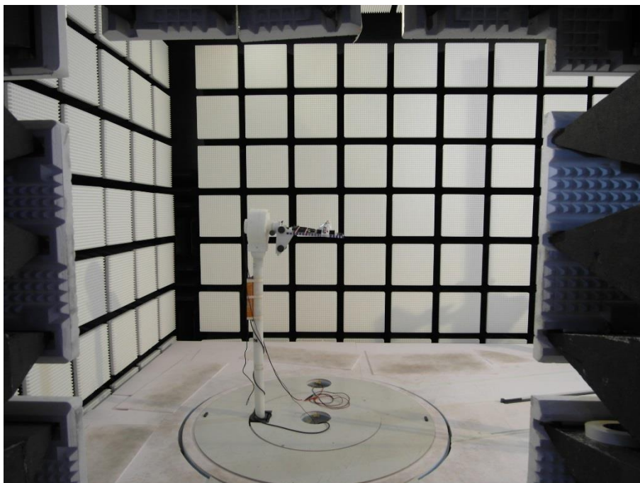
Photo 2: Fully Anechoic Chamber
