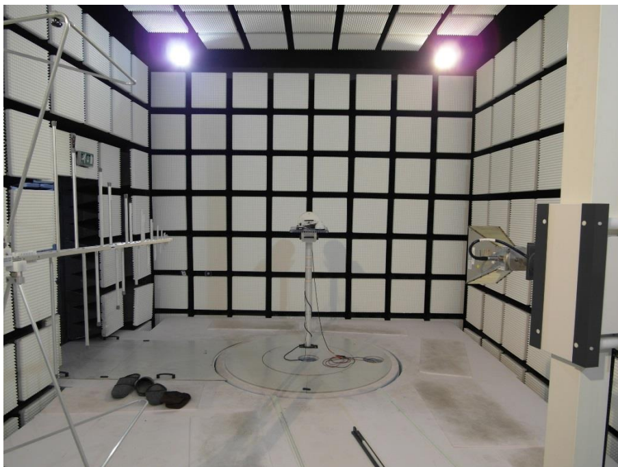
Photo 6: Fully Anechoic Chamber
