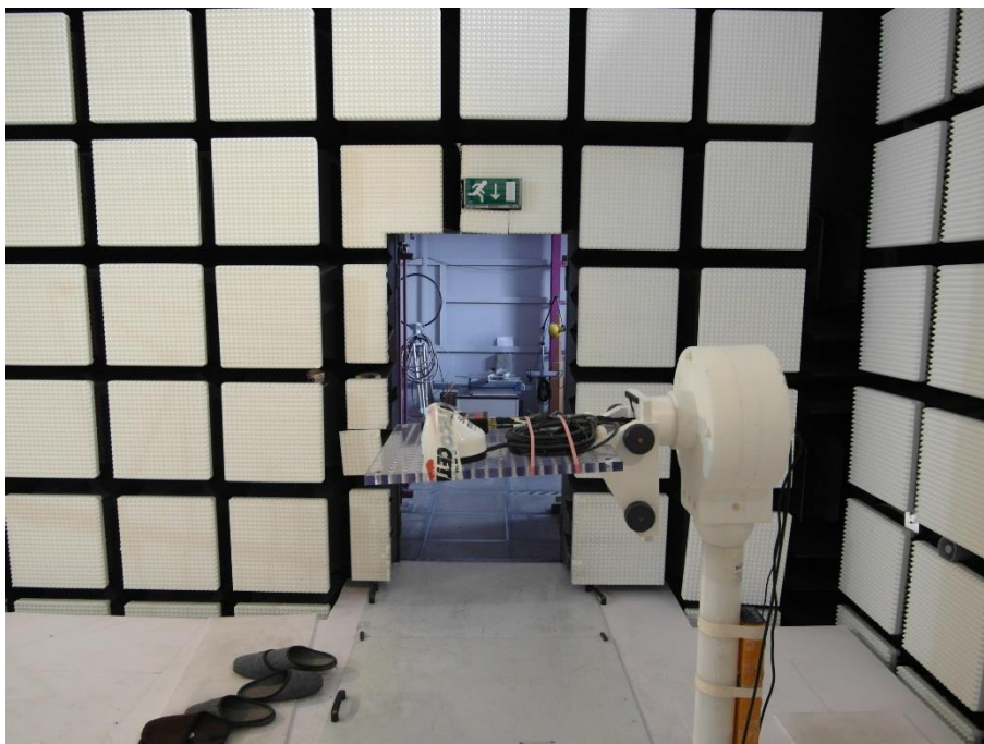
Photo 4: Fully Anechoic Chamber
