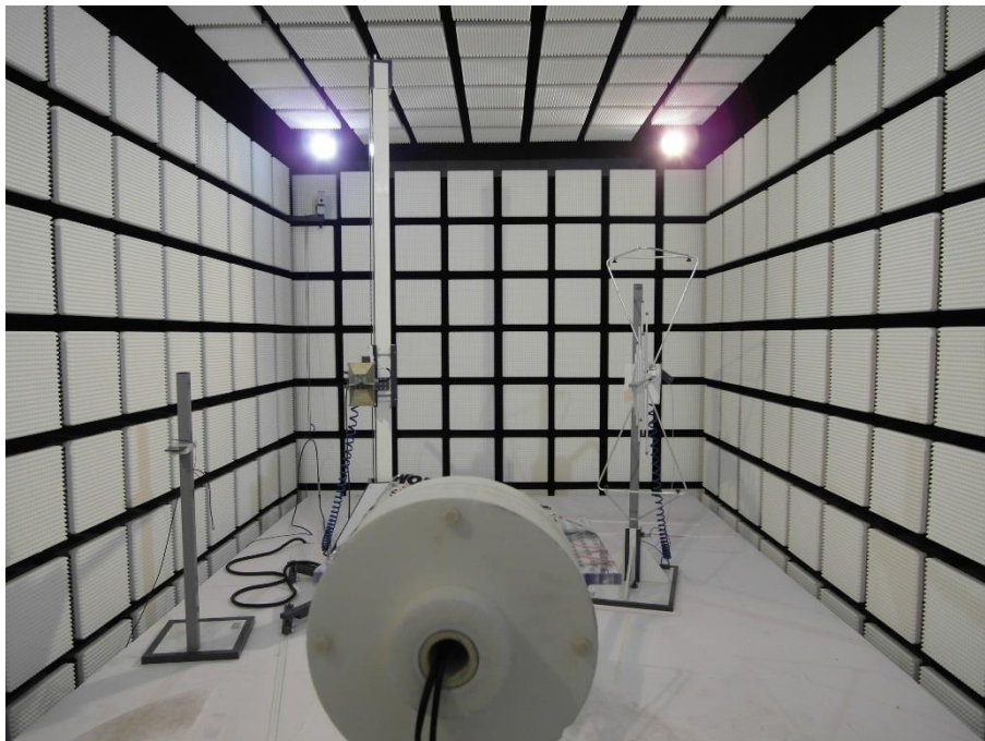
Photo 5: Fully Anechoic Chamber
