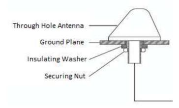
Vertical cut of a QF036 after installation
