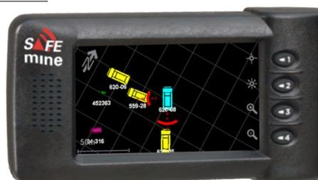
The ScopeScreen provides a 4" graphical display showing a bird-view map of the vehicle's surroundings. Its main use lies in rotational vehicles and stockpile applications which require detailed information on their environment. However SAFEmine strongly recommends the QD204 ScopeScreen to be installed with the QM105 Power Saving Display Cable connected to ignition, in order to preserve the vehicle battery from draining. Its installation is compulsory for light vehicles.
