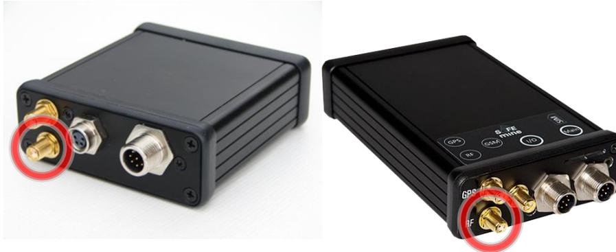
SAFEmine includes RF transceiver chips with typically less than 1% duty cycle and effective radiated power (ERP) is below 15mW. The CAS main units make use of the freely available industrial, scientific and medical (ISM) radio frequency bands for short range devices (SRD) and is thus license free. The transmission frequency of the system is software selectable by indicating the specific channel.
