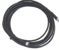
The QD221 and QD222 display extension cables provide 1.5m and 5m of cable in order to place the QD200 RemoteDisplay or QD204 ScopeScreen visible to the operator and remotely from the main CAS unit. The cable features a male and a female 4-pin plug with a pinout corresponding to the serial interface described in this chapter.
