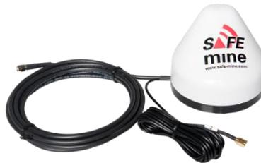
The magnetic mount antennas (QF024 GPS/RF, QF026 GPS/GSM and QF037 GPS/RF/WiFi) are equipped with a 3.5m pigtail of coaxial cable with 50Ω wave impedance. Its magnetic base attaches to any reasonably magnetic material. It allows an easy installation on vehicle roof tops and is ideal for light or other vehicles with moderate vibration.
