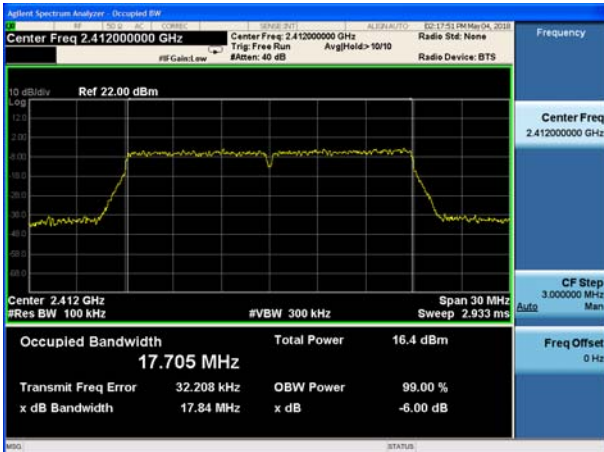
802.11n(HT20), Carrier frequency (MHz): 2437
