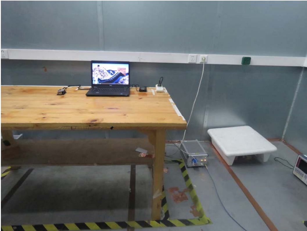
Picture 3 Conducted Emission Test Setup
