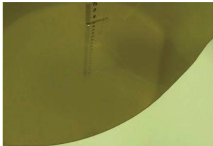
Picture 9.2-2: Liquid depth in the Flat Phantom ( Head 1750&1900 MHz )
