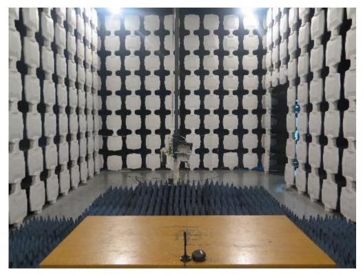
Pic2.Radiated emissions (1GHz-18GHz)
