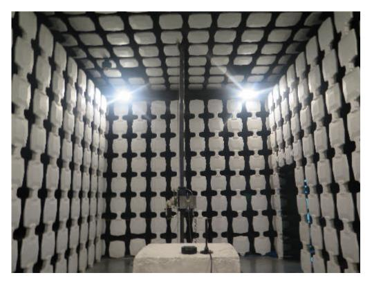
Pic3.Radiated spurious emissions (Above 1GHz)
