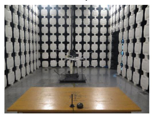
Pic1. Radiated emissions (30MHz-1GHz)
