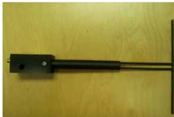
Figure 1 – MVG COMOSAR Validation Dipole
