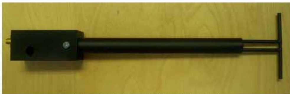
Figure 1 – MVG COMOSAR Validation Dipole
